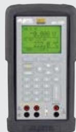
The MC-1200 Multifunction Calibrator provides the functions and accuracy associated with fixed-installations, laboratory instruments, and has everything needed for virtually any calibration task.
