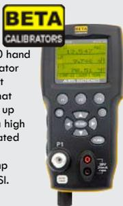
The BetaGauge 330 hand held pressure calibrator is a small lightweight calibration device that generates pressures up to 1.50 PSIG using a high performance integrated electric pump. Also internal manual pump version up to 300 PSI.
