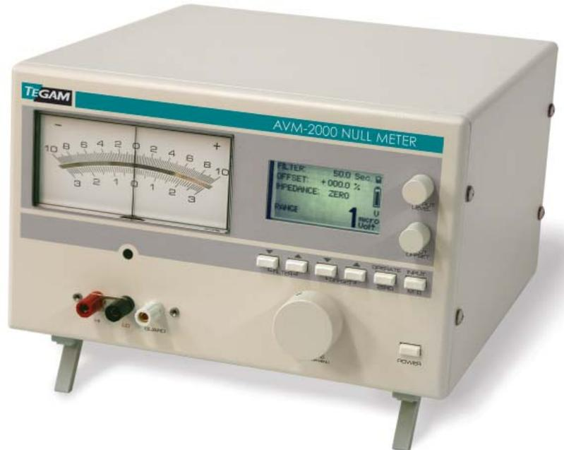
The Model AVM-2000 is a calibration laboratory grade Nullmeter/nanovoltmeter. It can be used as a stand-alone analog voltmeter or in conjunction with Kelvin-Varley dividers and other calibration laboratory equipment where high sensitivity ratio-metric processes are used.
