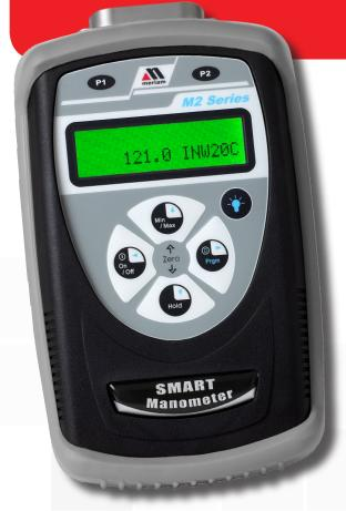
Meriam's M200LS Lab Standard Smart Manometer offers the best available pressure measurement accuracy in a portable, handheld format. The NIST traceable accuracy is typically  $\pm 0.01\%$  of F.S. and is independent of temperature effect over an operating temperature range of 59° to 86° F. Pressure ranges from 28" H<sub>2</sub>O F.S. to 500 PSIG F.S. are available.
